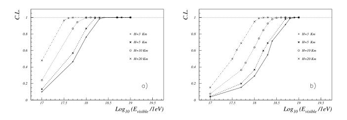
Fig. 1. Visibility confidence level of the second shower as function of its visible energy, at a simplified EUSO detector with efficiency 1 (left) and 0.1 (right), for horizontal showers at different heights. The horizontal dotted line shows the 99.7% CL  $(3\sigma)$ .
