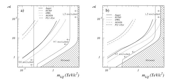
Fig. 4. Estimated sensitivities of the different cosmic ray experiments for scalar  $S_1$  (a) and vector  $V_2$  (b)  $1^{st}$  family leptoquarks, as a function of the leptoquark mass. The regions excluded by accelerator experiments are also shown for comparison. The observation times were taken as: 10 years for Auger, 3 years and 10% duty cycle for both EUSO and OWL. For AGASA and Fly's Eye, the exposure was taken from reference [16].
